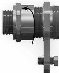
4. Locate the Armour Cone (3) into its recess in the Main Item (2). (N.B. For E1U and E2U variants, make sure the correct side of the cone is outermost - grooved for braid/tape armour and stepped for SWA). Pass the cable through sub-assembly "A" until the armour engaged with the cone. Spread the armour evenly around the cone.
