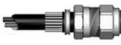
3. Ensure that the inner seal is relaxed by slackening the Main Item (2). Secure sub-assembly "A" into the equipment either by screwing the Entry Item (1) into a threaded hole or by securing it in a clearance hole using a locknut as applicable.
